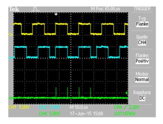
Here, two rising and two falling edges of the A and B signals (yellow and blue) are too close together, causing four alarm pulses (green). For each quantisation period in which an error occurs, one alarm pulse is issued.
