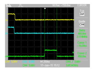
If the rotation speed is so high that A and B signals change within the same quantisation cycle (< 700 ns), resulting in missing 4x pulses, PR5201 triggers the Alarm pin. The screenshot shows an alarm-pulse due to a simultaneous A/B phase change. The pulse is typically 500 ns long. As Alarm is synchronized with the internal clock, the delay to the triggering event can vary, but is about 1.1 µs in this example.
