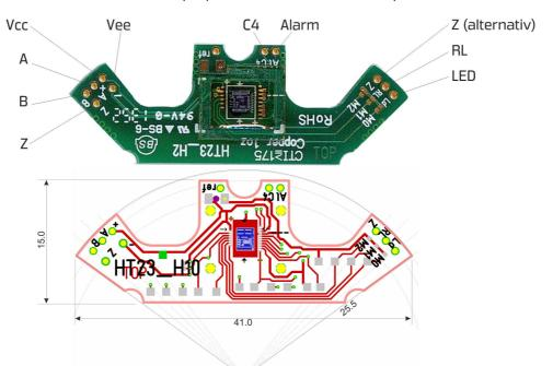
These images show a sample PCB for encoders with inner case diameter of at least 52 mm.
