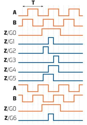
Remark: In mode **G6**, a proper Z pulse is achieved only with a disk with different phase between Z and A/B pattern than shown in the upper part of this image.
