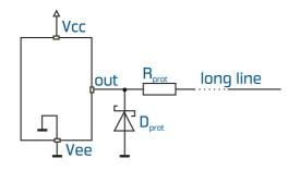
Recommended values are:  $R_{prot} > 50 \text{ Ohm}$  $D_{prot}$  type SD130B or equivalent (Schottky type)
