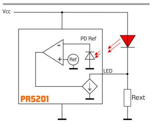
Especially at low supply voltage and when using LEDs with high forward voltage, the current driven by PR5201 may be insufficient. In this case a constant current can be added to the current regulated by PR5201, by connecting a resistor between the LED pin and Gnd. In this case, the LED current is given by:
