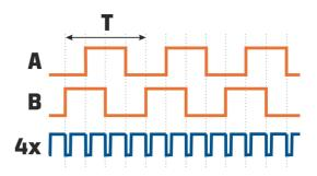
Due to the synchronisation, the 4x pulse can jitter within one quantisation period. In the example shown on the left, the minimum delay is 730 ns, the maximum is 1170 ns.
